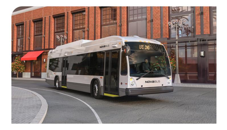
Smart technology powered by Nova Bus The LFS CNG is based on the proven LFS platform and integrates the latest in natural gas technology. Its rooftop catwalk is designed to facilitate maintenance and inspection.
